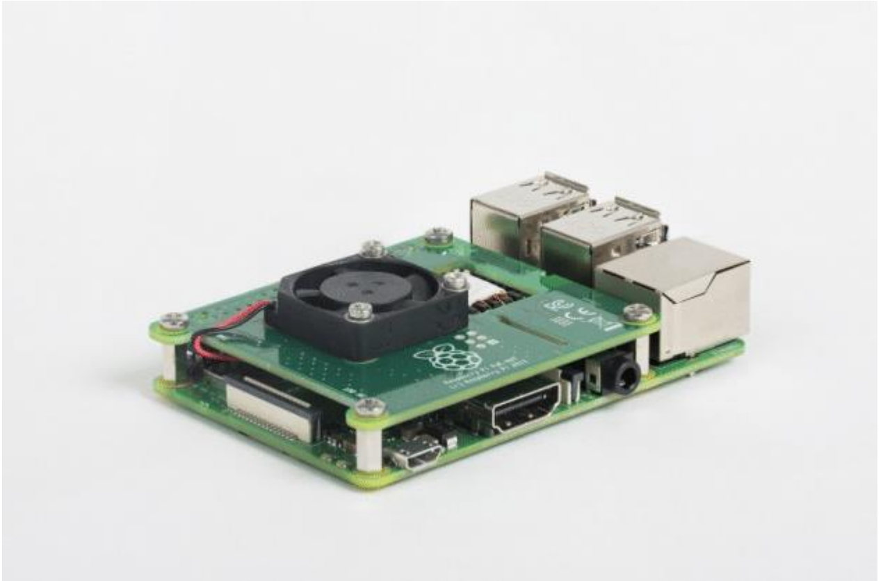
Figura 3: O Raspberry Pi PoE HAT e a nova Raspberry Pi 3 Modelo B+.
